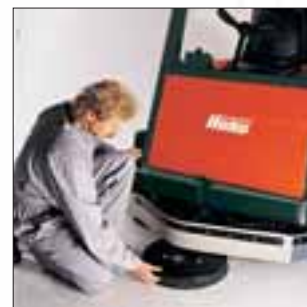
Quick brush change: In no time at all, without the use of tools.
