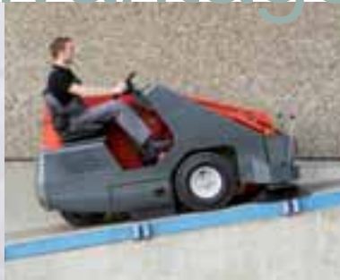
High climbing ability: thanks to the hydraulic drive gradients of up to 16% can be negotiated without problem, whilst sweeping.
