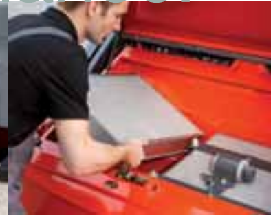
High degree of separation of over 99%. The large filter surface area of more than 11m 2 separates the dust cleanly from the air.
