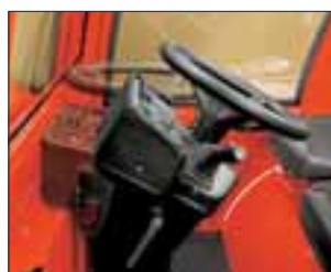
Adjustable steering column – relaxed driving position.
